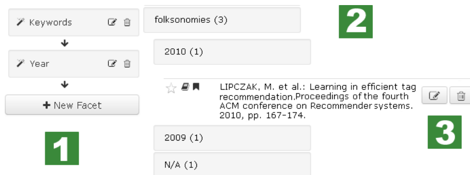
Fig. 1. Example of a facet tree hierarchy, with Keywords and Year facets selected (1). Folder with keyword folksonomies (2) is expanded showing three subfolders containing also NA value. User can edit the resource and its metadata or remove it from the collection (3).
