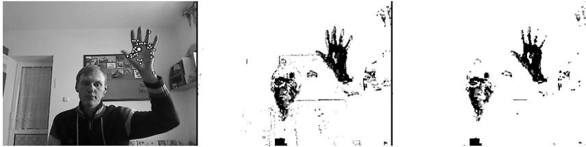
Figure 3: Original image with flock of features, result of histogram back projection with noise, removing noise with operation open (erosion and dilatation) [1].
