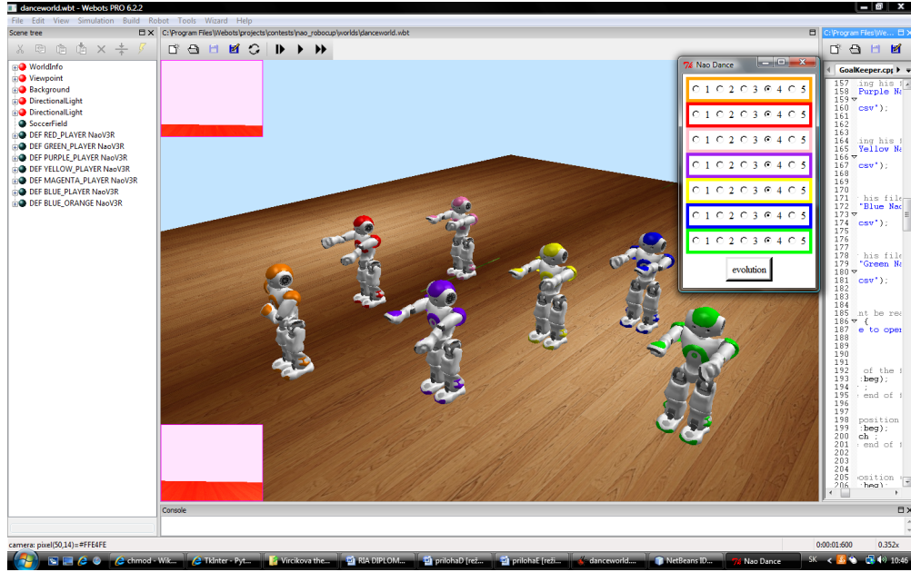
Fig. 3. Our user-interface for simulation of robotic dances in Webots and connected with evolutionary algorithm in programming language Python. User interactively co-operates with the system evaluating the showed dancing performance of each robot and gives them marks according to his own opinion and preferences.
